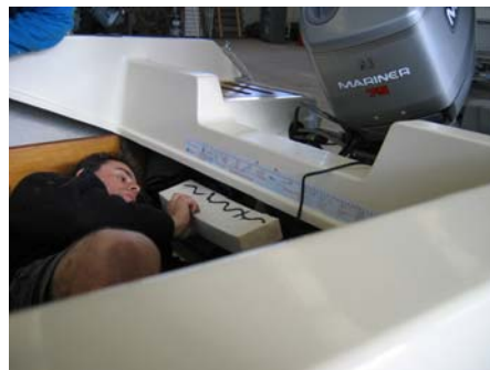
Foam being fitted under the outboard well with Sikaflex
