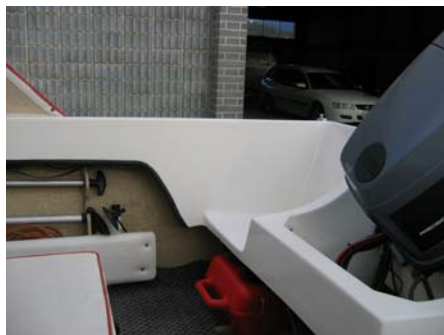
Foam can be fitted under the outboard well and deck mould
